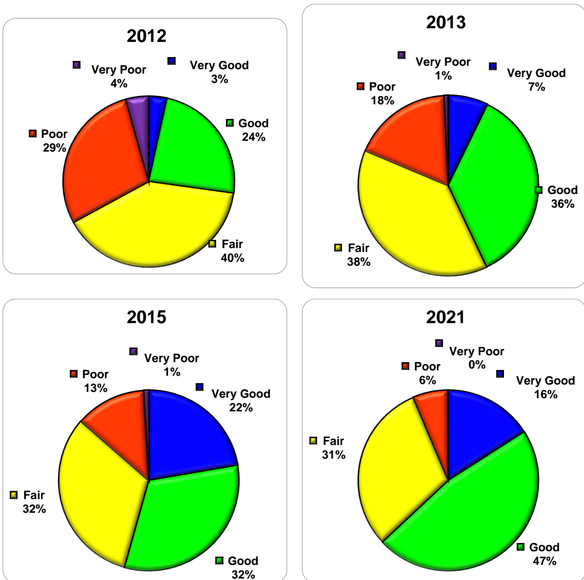
Figure 4: Historic and current average VCI condition distribution over the last decade.
